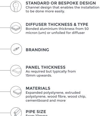
**PANEL THICKNESS** As required but typically from 15mm upwards.
